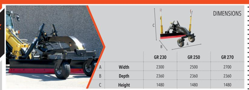
The Grader Blade M3 can be fitted to the small skid steer loaders with power ranging from 50 to 120 HP is ideal for the preparation and the leveling of lands, roads and yards. It is equipped with the tilt system 32°, oscillation 40° and translation 450 mm of the blade through an hydraulically controlled push button, manual flow regulator on the distributor on / off, ST52 steel structure, attachment to the machine, hydraulic hoses and electric control kit.
